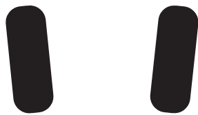
Negative camber where the top of the wheel points out
