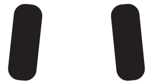
Positive camber where the top of the wheel points in
