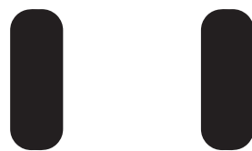
Zero camber Where wheels are parrallel
